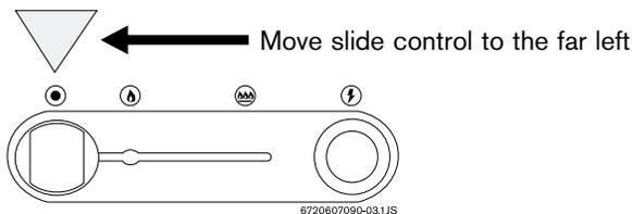
Fig. 15 - Gas control slide - shut down position
