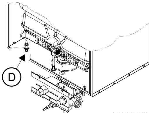
Fig. 16 - Burner pressure test point
