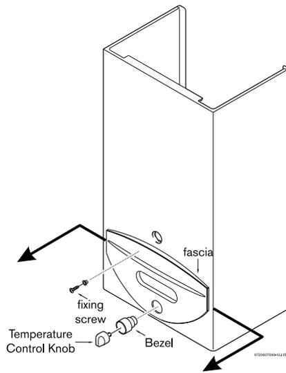
Fig. 17 - Access for servicing
