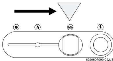
Fig. 14 - Gas control slide - operating position
