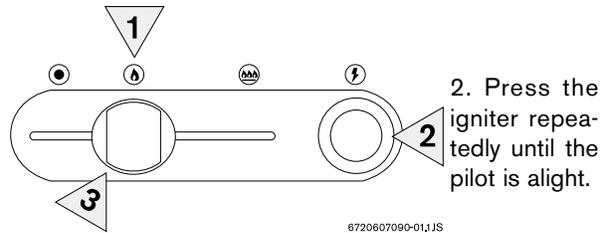
3. Release the slide control approx 10 seconds after pilot lights.
