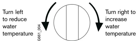
Note: with higher temperatures the available flow of water will be reduced.
